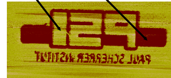
Chemical patterns after lift-off: LFM image
