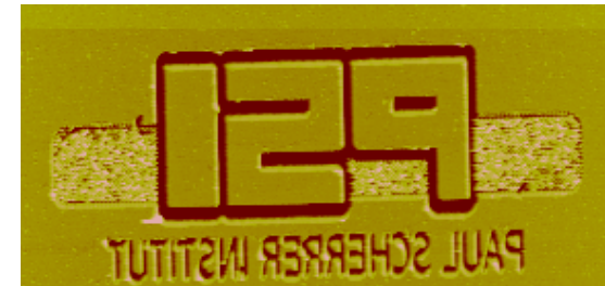
Embossed structure: AFM image
